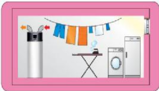
Dehumidification in the recirculating air
